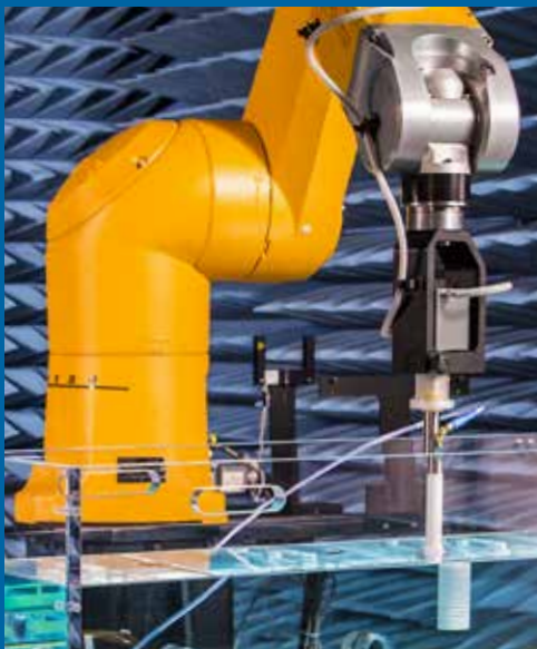
Scanning in progress with DASY52NEO (SPEAG, Switzerland)
