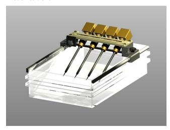
A probe positioner made of PMMA has been developed for the phantom. This positioner can be adjusted along 3 axes, allowing accurate positioning of all **SPEAG** probes. The compatible field probes include E-field, H-field, dosimetry (SAR) and temperature probes and can be used inside a clinical MRI scanner. The positioner enables repeatable measurements in the empty and liquid filled phantom of  $\pm 2$ mm.
