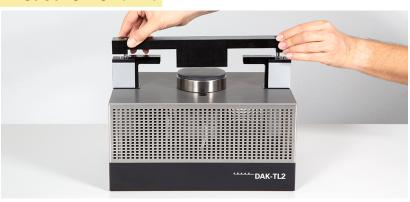
This new product is based on an innovation of the computational electromagnetic group of the IT'IS Foundation, namely a novel high-performance solver that directly determines the dielectric parameters from measured  $S_{\rm 11}$  values in quasi real time – instead of using precomputed lookup tables. This makes the system not only more precise but also more flexible.
