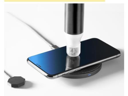
The full version 1.0 of cDASY6/8 Module WPT, designed to demonstrate compliance with the basic restrictions of any magnetic source from 3 kHz to 4 MHz with maximal precision, has now been released. It is fully compliant with IEC/IEEE63184 PAS and empowers manufacturers to certify devices with minimal overestimation (up to 70 dB more currents than if compared to the reference levels).
