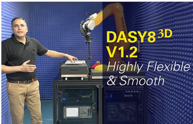
SPEAG released two new versions of DASY that significantly improve the automation of specific absorption rate (SAR) testing (DASY8<sup>3D</sup>) and that of the assessment of the incident power for distances smaller than  $\lambda/5$  (Module mmWave). The latter has already been adopted by regulators. Learn about the main new DASY8<sup>3D</sup> features in this short user [video](#).
