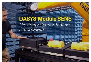
SPEAG has released DASY8 Module SENS V1.0 $\beta$ , a system designed for automated standards-compatible testing of proximity sensors – including the latest time-averaged proximity sensors – of wireless devices. The module is based on a research collaboration, supported by Innosuisse, between the IT'IS Foundation and Semtech. See a demonstration of DASY8 Module SENS in action by watching our <u>video</u>.
